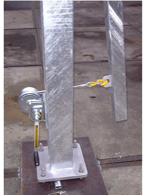
Detail removable winch for rising and lowering pole.
